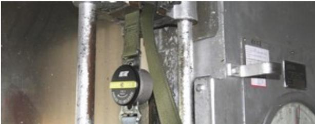
We suspended a QRB Mk-3 in the test bench equipped with normal standard fork tangs between 2 pieces of type XIII webbing. It was extremely exiting to observe the test run.
