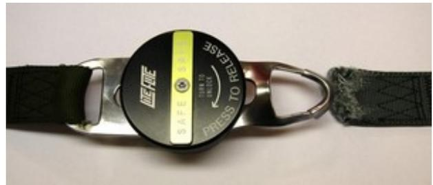
The most interesting result of the test was that the QRB itself did not suffer any harm and the mechanism functioned flawlessly afterwards. It showed no sign of any damage after a pull test to 2.54 tons. Amazing.
