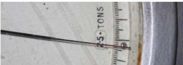
At 1.3 tons the webbing slots in the two tangs began to deformate. Except from the effect of the
